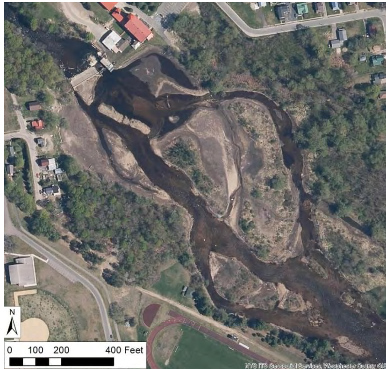
Photo 4-5 2020 NYS orthophoto showing sediment aggradation at Ballards dam
