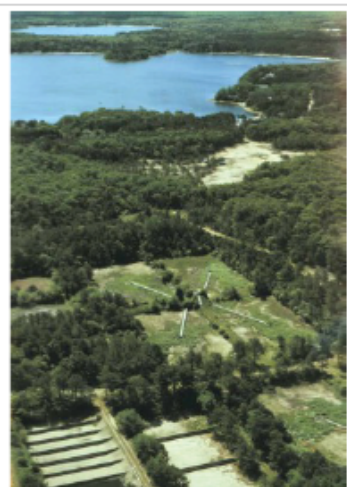
Treated wastewater from Joint Base Cape Cod was discharged to rapid-infiltration disposal beds from 1936 to 1995. The disposal formed a groundwater contamination plume that extends more than 10 kilometers in the Cape Cod sand and gravel glacial outwash aquifer. Photo credit: Denis R. LeBlanc, USGS
